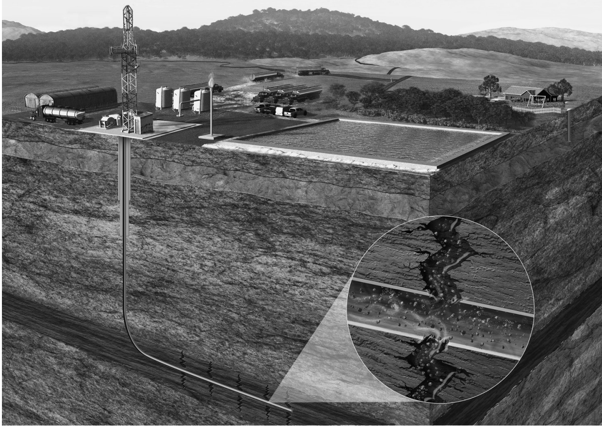
Hydraulic fracturing creates pathways for oil and gas to flow from shale and other types of compressed rock.
